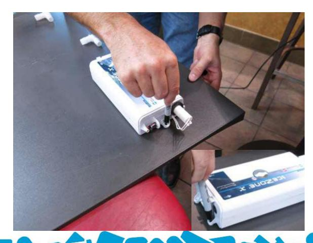
Drill the holes to mount the XSafe<sup>®</sup> Unit on the lid.
