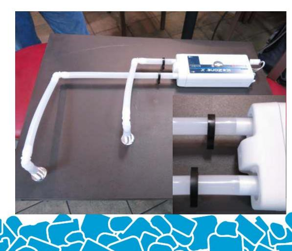
Tighten the handy clamps with a pliers to secure the tubing on the XSafe<sup>®</sup> unit.
